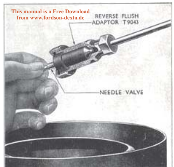
Fig. 29 Reverse Washing the Nozzle
