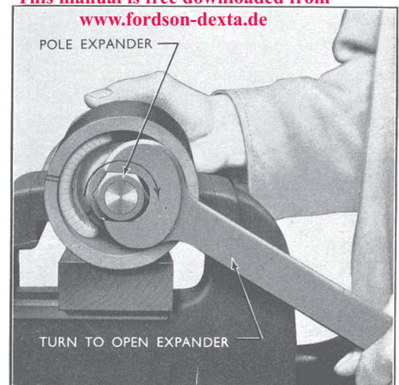
Fig. 6 Expanding the Pole Pieces
