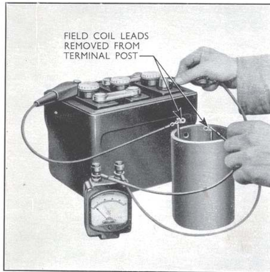
Fig. 5 Testing Field Coils for Continuity
