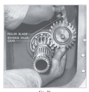
Fig. 30 Checking Reverse Idler Gear End-float
